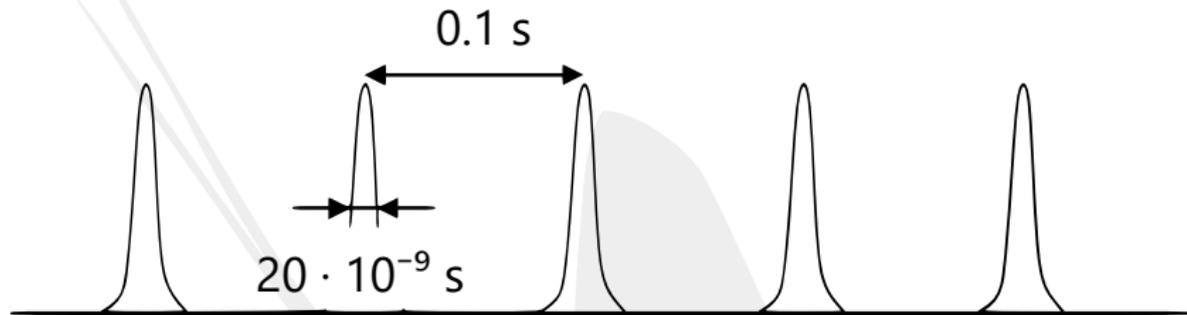
**EG** Nd-YAG laser with repetition rate  $f = 10 \text{ Hz}$ , pulse energy  $E = 2 \text{ J}$ , pulse duration  $\tau = 20 \text{ ns}$
