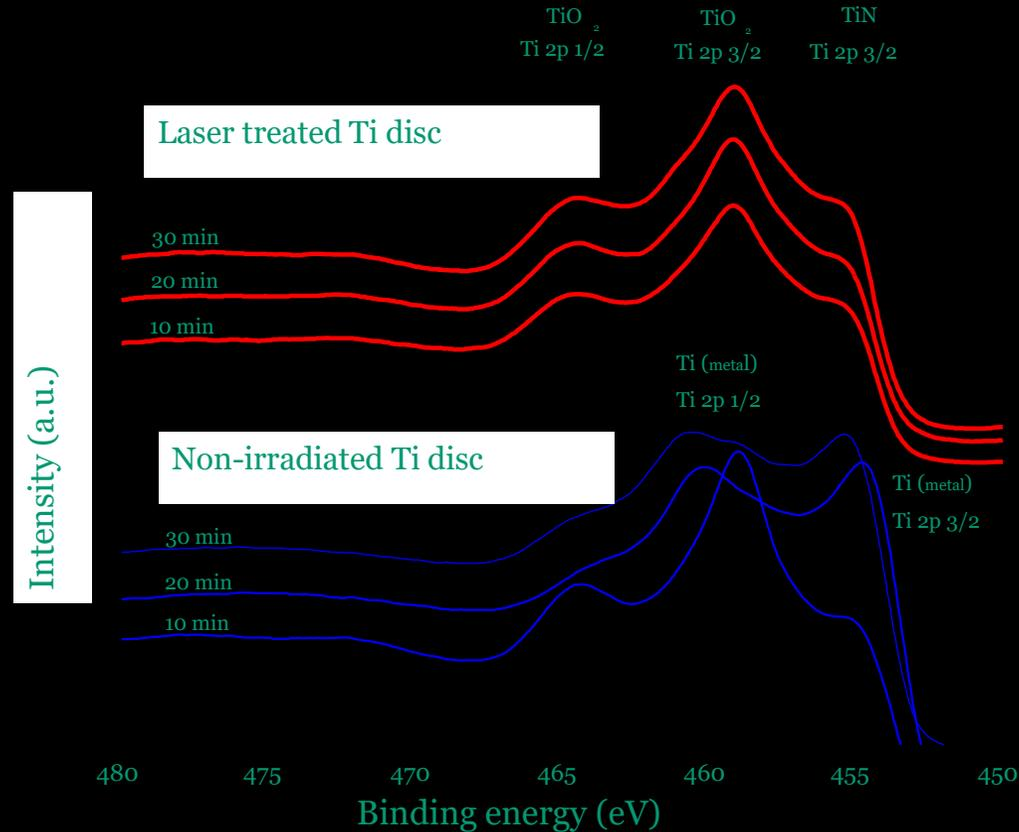
increased the thickness of the TiO<sub>2</sub> layer.
