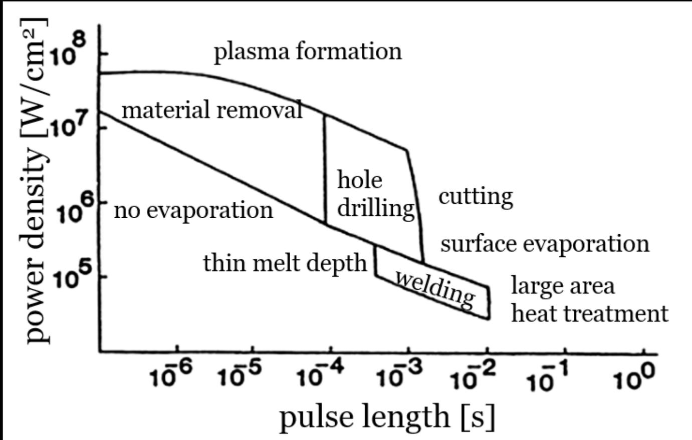
1. Heat treatment: Condition near to melting point temperature. This is achieved with low power density ( $\text{kW}/\text{cm}^2$ ) and high pulse length ( $> 10^{-2}$  s).
