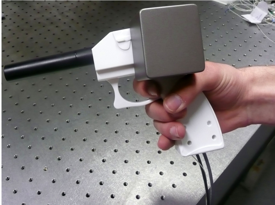
Hand held 1D lateral scanner with extended focus to access internal parts of the mouth
